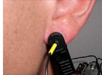
Leave enough slack in the cable to allow the patient to turn their head easily, but not too much that it can get caught. Think about the angle of the cable from the ear clip to the neck clip, so that no extra tension is placed on the ear clip.
