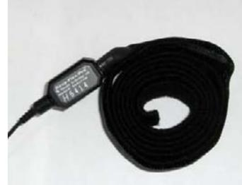
Unravel the strap and attach it around the abdomen so that the sensor is in the front. The fit should be snug enough that the strap stays fixed when the subject is relaxed.
