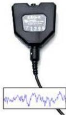
The EEG-Z is a pre-amplified electroencephalograph sensor with built in impedance sensing capabilities. This sensor can be toggled to record regular EEG or monitor skin impedance (both the reactive and resistive elements) to help optimize electrode hook-up.
