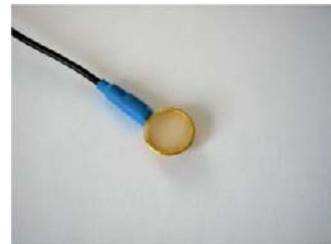
Add more Ten20 paste onto the cup electrode, just enough to form a ball on the cup, not so much that it spills over the edge. Shown is the ideal amount of paste.
