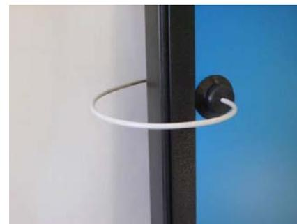
4. Insert the other end of the fiber optic cable into the AV Sync sensor.
