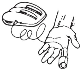
3. Wrap the Velcro® around your finger or toe to hold the sensor in place, using only enough pressure to hold it there. Do not apply pressure or inaccurate readings may result.
